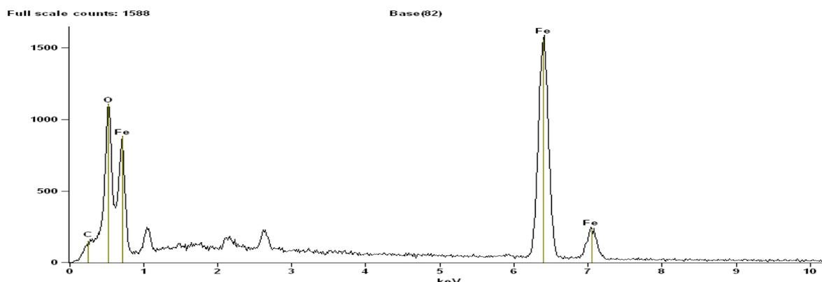
FIG 4: EDAX analysis of the starch stabilized nZVI
