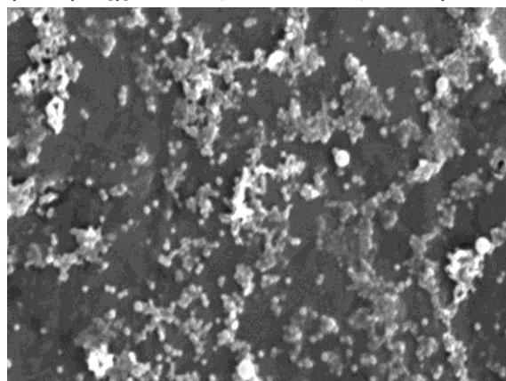
FIG 3: SEM image of the Starch stabilized nZVI
