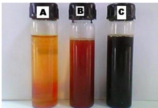
Fig 1: colour change during green NZVI synthesis (A- Fe(NO<sub>3</sub>)<sub>3</sub> solution , B-tea extract, C-NZVI)
